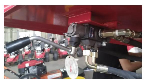
By operating the handle, there are 3 functions of the feeding roller: Feeding, Reversing, hold-on.
