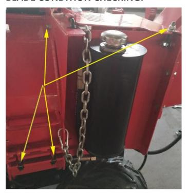
By Loosing these 4 bolts, can open the chamber to check the condition of blades and fans.
