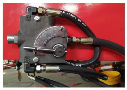
The bar can adjust the rotating speed of the feeding roller(from 0-600RPM).
